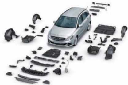
FIGUUR 19: GERECYCLEDE KUNSTSTOFFEN IN DE MERCEDES B-CLASS ELECTRIC DRIVE (BRON: MERCEDES-BENZ)
