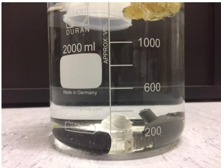
Figure 3: Sealants and plastic parts in water: Floating: PE cap and polyurethane sealant. Sinking: MS Polymer sealant (black), Acrylic sealant (grey) and silicone sealant (white).
