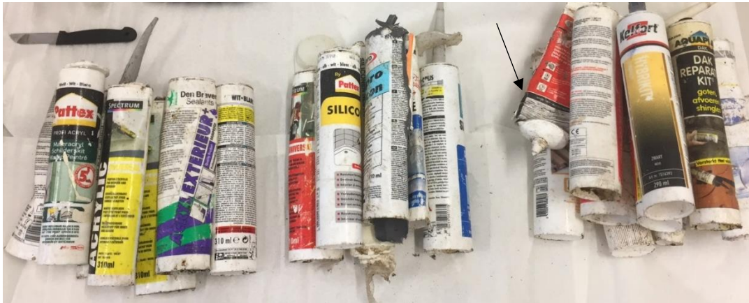
Figure 1: Sealants, sorted by type of sealant. Left: acrylic. Middle: silicone. Right: Construction sealants (mainly MS polymer) and others.
