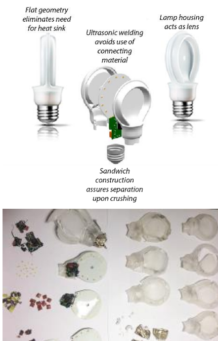
FIGURE 32: PHILIPS SLIMSTYLE LED. TOP: DESIGN CHOICES WITH REFERENCE TO RECYCLABILITY. BOTTOM: SHREDDED SLIMSTYLE LEDS (SOURCE: PHILIPS)
