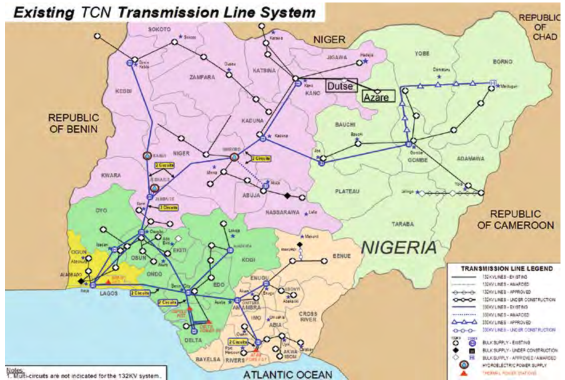
Figure 2.13 Existing Transmission Line System (Transmission Company of Nigeria, 30 June 2015)
