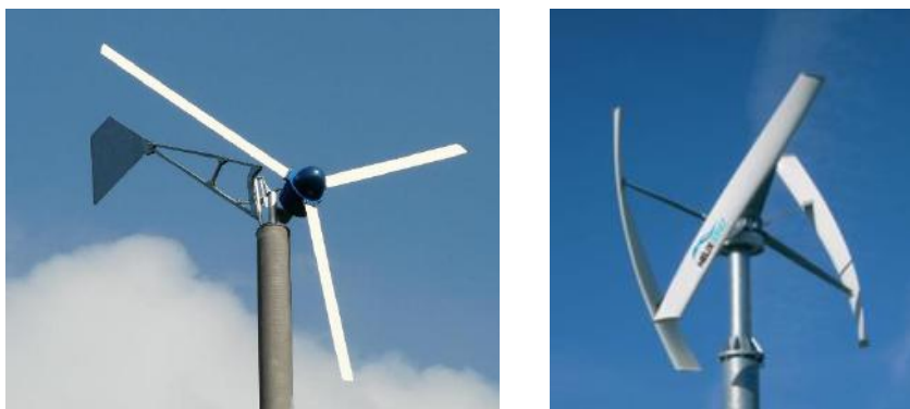
Figure 10: Horizontal axis wind turbine (left) and vertical axis wind turbine (right)
